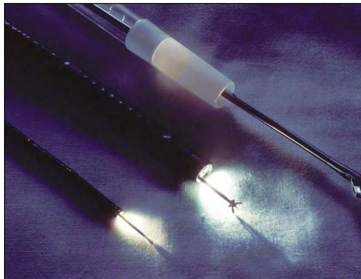
Light emitting diodes used together with ex. highspeed endocam.
